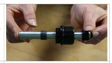
Carefully grease all components, the gear ring in the hub housing, the seals and the surface of the bearings with fluid grease especially between pawls and their sliding surfaces on the freewheel body.
