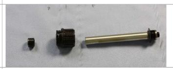
Clean and degrease the toothing in the hub body and the axle. Use a soft cloth and a gentle degreaser. (Isopropanol)
