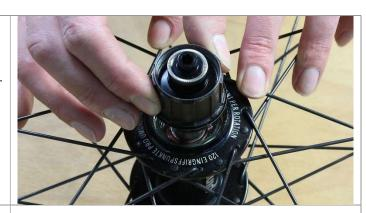
Pull the spacer sleeve and freewheel body off the axle - if necessary, tap lightly with a plastic mallet.
