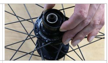
Tighten the lock ring with an HG tool 40Nm 30ft-lb
