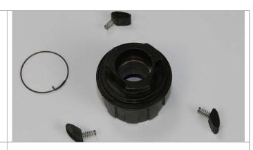
Insert pawls and springs into the freewheel body in the correct position.
